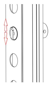
**Connector orientation:** foot is aligned up and down (x3)
