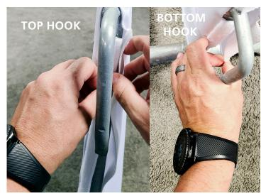
Pull graphic across frame and down the second side of your barricade. Smooth out any wrinkles. Insert top and bottom barricade hooks into the slits in the graphic.
