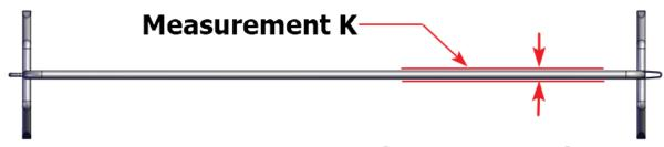
Measurement K- Measure diameter or thickness of frame tube as shown below.
